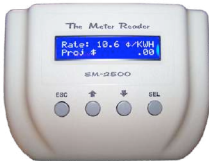
Figure 27. Energy Monitoring Technologies Meter Reader display
