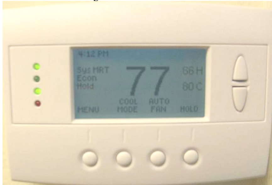
Figure 63. Programmable Communicating Thermostat Showing Current Settings During a Tier 4 Price Event
